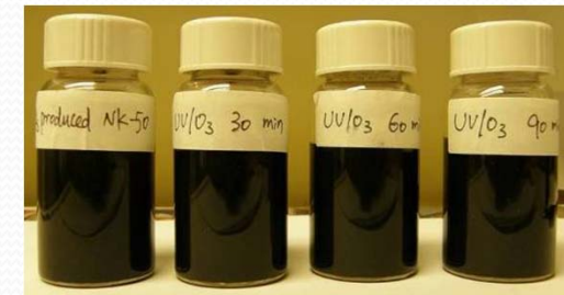
24 h after sonication CNT-C in ethanol for 30 S; C_{\text{CNT}} = 0.2 mg/mL.
